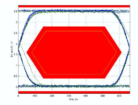
Figure 10. Low Speed Signal Quality Eye Diagram Test (NLAS7222A with  $V_{CC}$  = 3.6 V)
