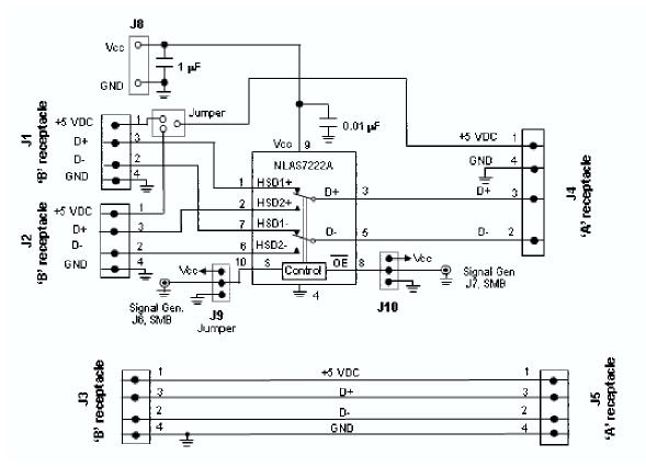
Figure 7. Schematic of the NLAS7222A USB Demo Board
