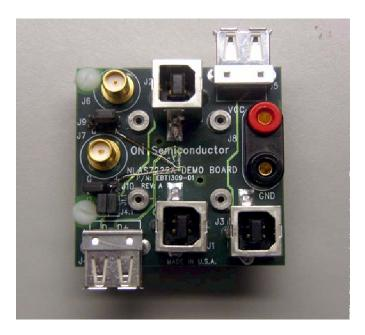
Figure 9. Photograph of the NLAS7222A USB Demo Board
