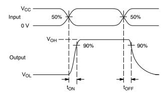
Figure 3. t<sub>ON</sub>/t<sub>OFF</sub>
