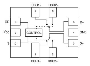
Figure 1. Pin Connections and Logic Diagram (Top View)
