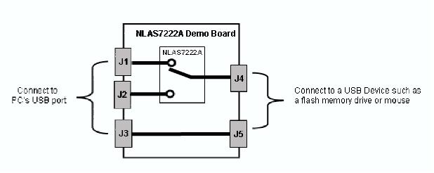
Figure 8. Block Diagram of the NLAS7222A USB Demo Board
