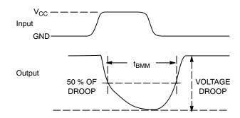
Figure 2. t<sub>BBM</sub> (Time Break-Before-Make)
