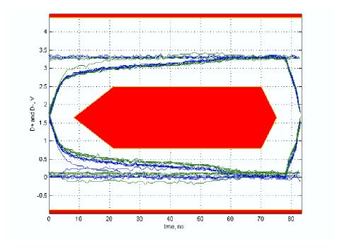
Figure 11. Full Speed Signal Quality Eye Diagram Test (NLAS7222A with  $V_{CC}$  = 3.6 V)
