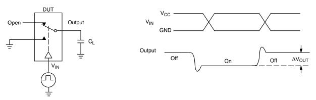
Figure 6. Charge Injection: (Q)
