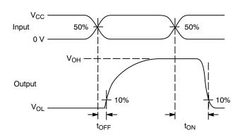
Figure 4. t<sub>ON</sub>/t<sub>OFF</sub>
