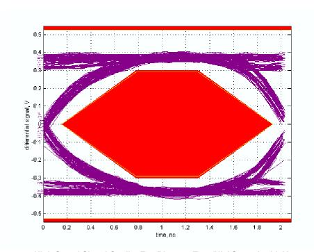
Figure 12. High Speed Signal Quality Eye Diagram Test (NLAS7222A with  $V_{CC}$  = 3.0 V)
